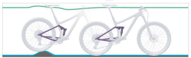
Figure 149: Optimum rear frame damper ride performance over bumps
