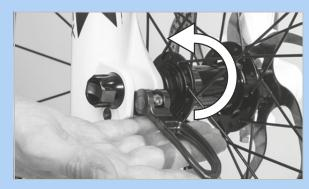
Figure 75: Pressing the quick release lever in the direction of the arrow
