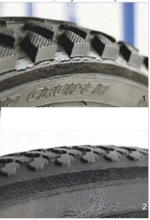
Figure 167: Examples of fatigue cracks (1) and ageing cracks (2)
