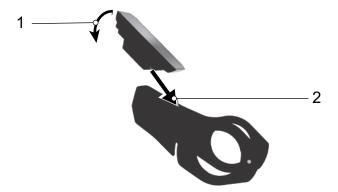
Figure 128: Inserting the display
