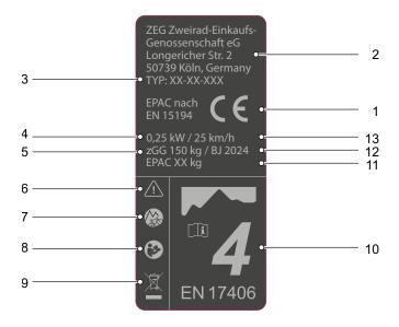
Figure 2: Example of ZEG nameplate
