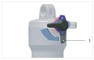
Figure 146: The compression adjuster's (black) open position (1)
