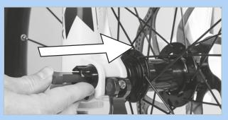
Figure 74: Pushing the red lever in the direction of the arrow
