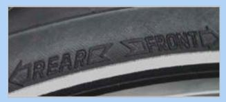
Figure 67: Rotation direction arrow on MTB tyres
