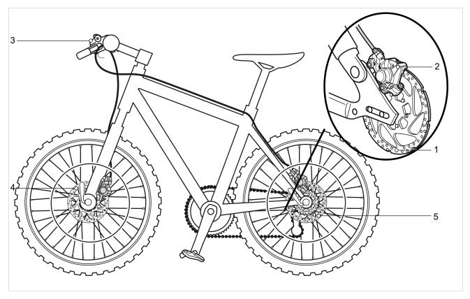
Figure 35: Brake system with disc brake - example
