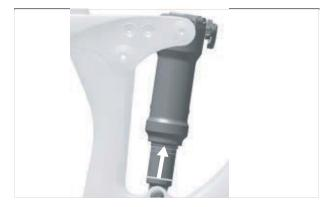
Figure 122: Moving the O-ring on the rear frame damper
