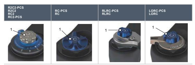
Table 134: Low-speed lever (1) on the SR Suntour suspension fork on the fork crown
