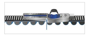
Figure 174: Check gauge on belt
