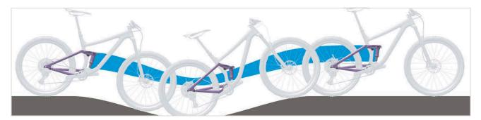
Figure 201: Excessively soft suspension in the rear frame damper on hilly terrain
