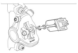
Figure 65: Fastening the transport securing device
