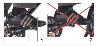
Figure 141: Correct (1) and incorrect (2) foot position on the pedal
