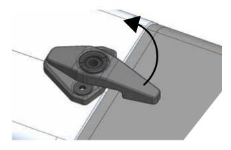
Figure 135: Opening the locking lever
