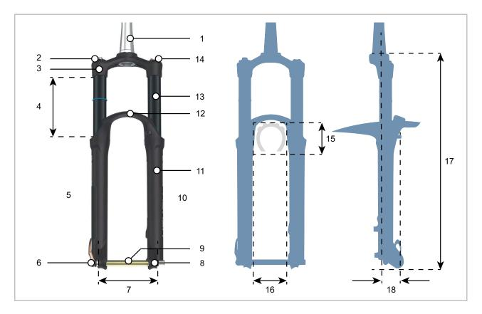
Figure 13: Parts of a suspension fork
