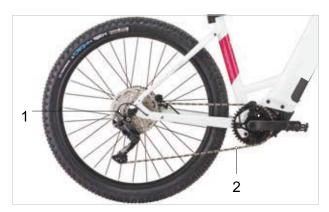
Figure 45: Chain drive with derailleur gears
