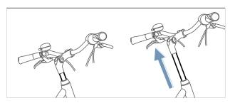
Figure 105: Adjusting the quill stem height
