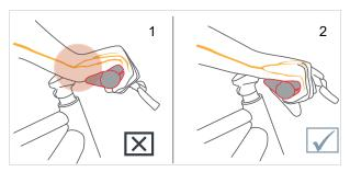
Figure 109: Incorrect (1) and correct (2) position of the handle
