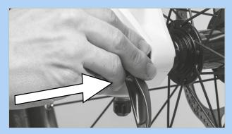
Figure 79: Inserting the quick release in the direction of the arrow
