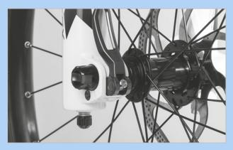
Figure 186: Adjusting the quick release clamping force
