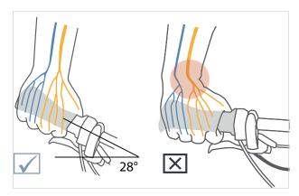
Figure 102: Distribution of nerves with curved and straight handlebars
