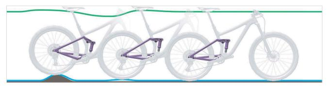
Figure 197: Rear frame damper rebounding too quickly
