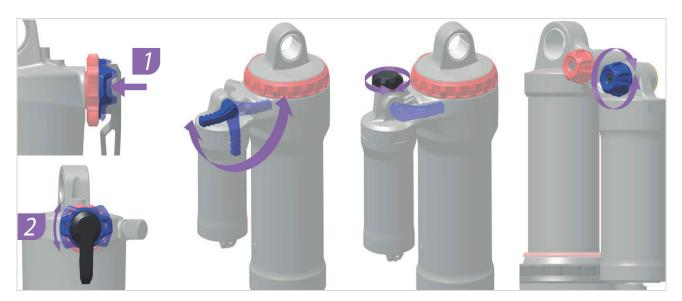
Figure 202: Position and shape of the compression adjuster (blue) depends on the model
