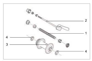
Figure 32: Example of front wheel hub: SHIMANO
