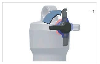
Figure 145: The compression adjuster's (black) closed position (1)
