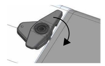
Figure 136: Closing the locking lever
