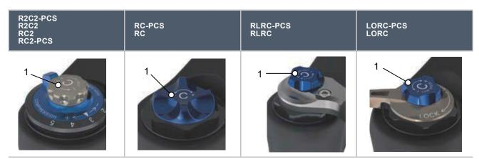
Table 133: Low-speed lever (1) on the SR Suntour suspension fork on the fork crown
