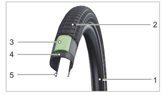
Figure 26: Structure of tube-type tyre
