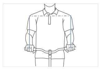
Figure 101: Determining the optimal handlebar width
