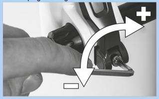
Figure 187: Adjusting the quick release clamping force
