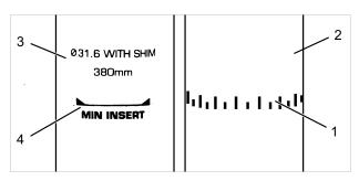
Figure 98: Detailed view of the seat post – examples of the minimum insertion depth marking
