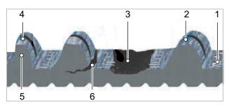
Figure 169: Indications of wear on a belt
