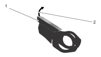
Figure 130: Removing the display
