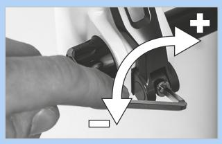
Figure 77: Adjusting the quick release clamping force
