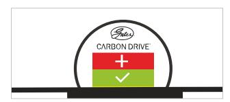
Figure 179: Example: On yellow along lower edge, so reduce belt tension slightly
