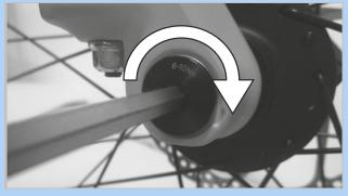
Figure 69: Tighten the axle in the direction of the arrow
