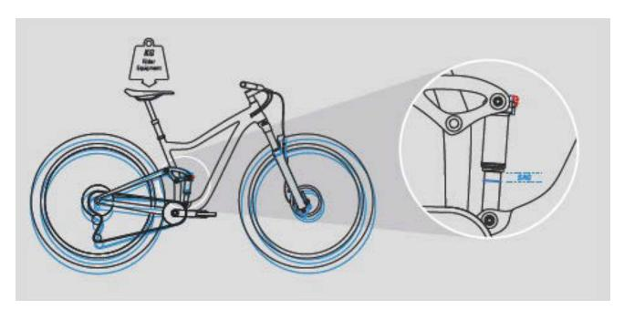
Figure 120: SAG rear frame damper
