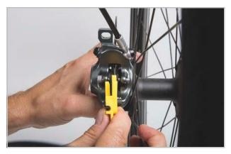
Figure 168: Checking the brake lining when fitted with the help of the transport safety wear gauge
