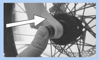
Figure 68: Inserting the axle in the direction of the arrow
