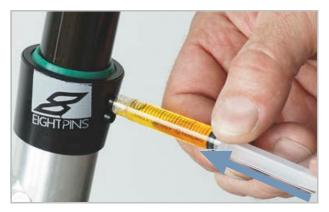
Figure 164: Lubricating the Eightpins seat post
