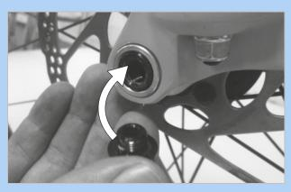
Figure 70: Inserting the securing screw
