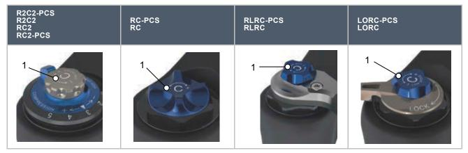
Table 119: Low-speed lever (1) on the fork crown on the SR Suntour suspension fork
