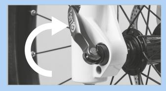
Figure 81: Closing the quick release
