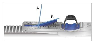
Figure 176: Example of a reading: 20 kg
