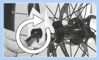
Figure 73: Tighten the axle in the direction of the arrow
