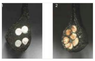
Figure 27: Steel bead core (1) and Kevlar bead core (2)
