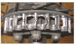
Figure 172: Photo showing example of worn tooth profile
