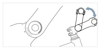
Figure 107: Different versions of angle-adjustable stems
