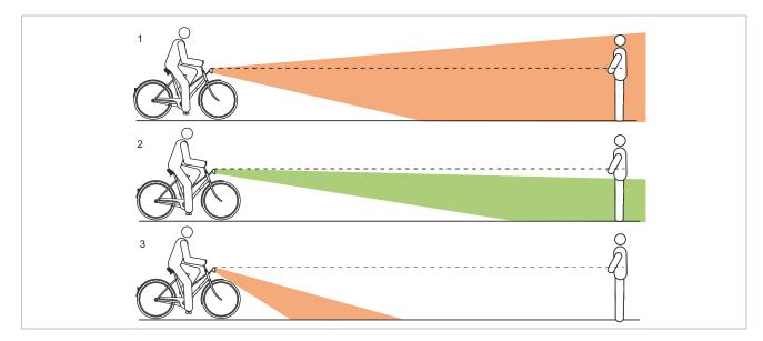
Figure 125: Light positioned too high (1), correctly (2) and too low (3)
