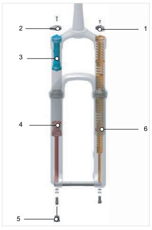
Figure 15: Internal structure of a steel suspension fork
