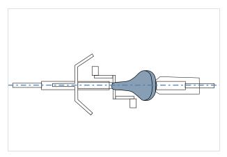
Figure 95: Positioning the saddle in direction of travel
