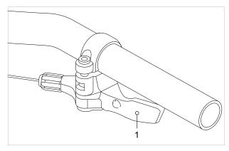
Figure 142: Remote control operating lever (1)
