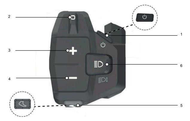
Figure 53: Overview of the BOSCH control panel
