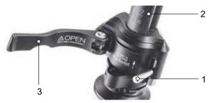
Figure 82: Opened clamping lever on the stem quick release (3) on the stem (2), version I, with locking lever on the stem (1)
