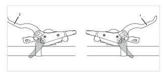
Figure 153: Handbrake, front (2) and rear (1) – SHIMANO brake used as an example
