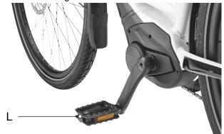
Figure 85: L pedal in the left-hand crank arm
