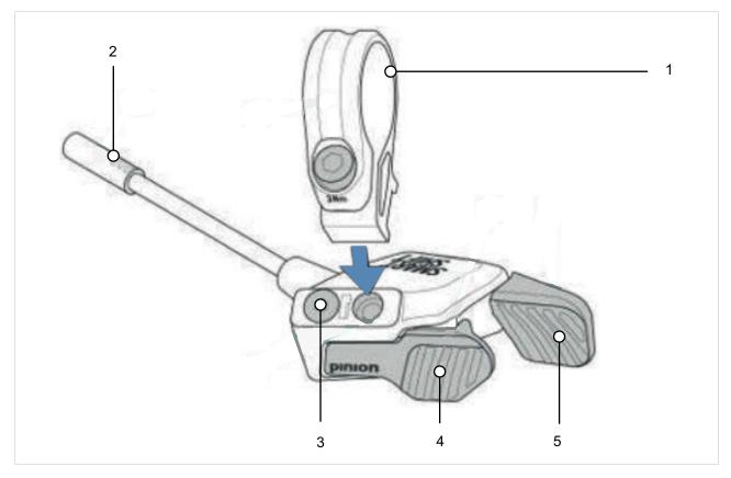
Figure 62: Parts of Pinion E-Trigger TE1
