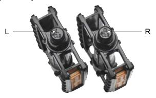
Figure 84: Example of markings on pedals
