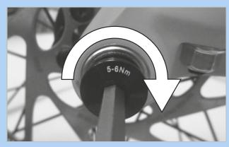
Figure 71: Tightening the securing screw
