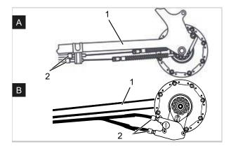
Figure 184: Adjusting sleeves (2) on two alternative versions (A and B) of a dual-cable, Bowden-cable-operated gear shift on the chain stay (1)
