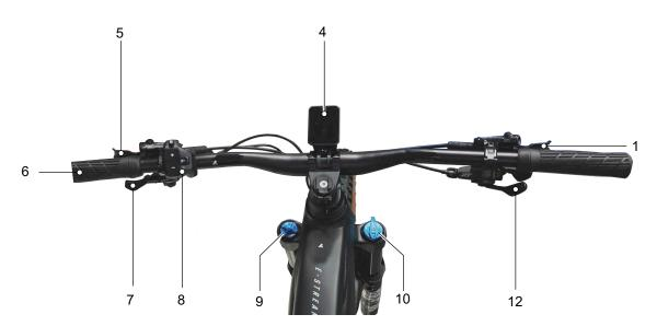
Figure 52: Detailed view of handlebars with FIT Remote Basic on-board computer and Compact 2.0 display
