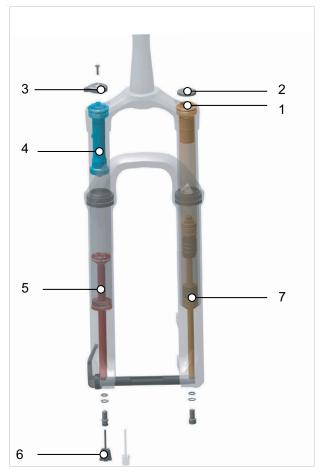
Figure 14: Internal structure of an air suspension fork
