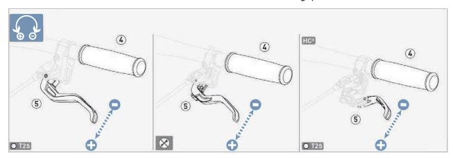
Figure 117: Adjusting the grip distance for a MAGURA handbrake disc brake
