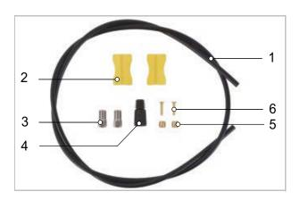
Figure 34: Components in a brake cable
