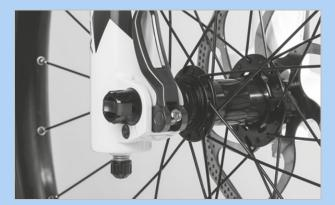
Figure 76: Perfect position for the clamping lever
