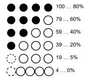
Table 97: Battery level indicator when discharging
