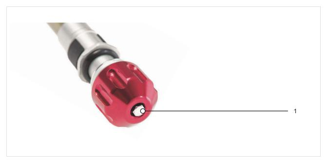
Figure 123: Example of SR SUNTOUR rebound adjuster (suspension fork) (1)
