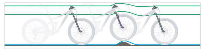
Figure 196: Excessively hard damping in the suspension fork on bumps
