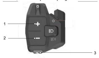
Figure 152: Position of plus button (1), minus button (2) and push assist button (3)
