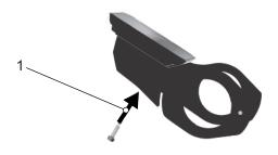
Figure 129: Fastening the blocking screw
