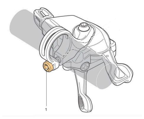
Figure 118: Position of attachment screw (1)
