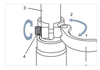
Figure 97: Opening the seat post quick release
