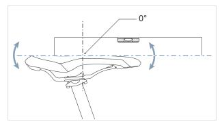
Figure 100: Horizontal saddle tilt with 0° tilt in the centre of the saddle
