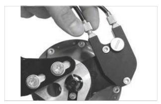
Figure 183: The tension adjuster on ROHLOFF hub versions with external switch control is located on the cable box positioned on the left-hand side
