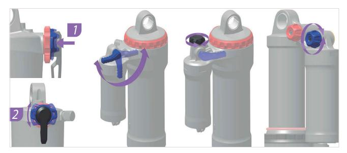
Figure 204: Position and shape of the compression adjuster (blue) depends on the model
