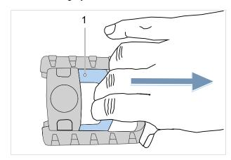
Figure 161: Pulling the pedal folding latch (1) downwards
