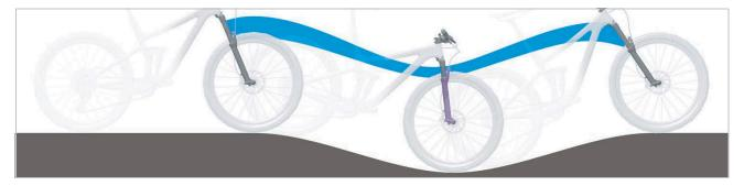
Figure 195: Excessively soft suspension in the suspension fork on hilly terrain
