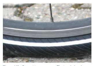
Figure 110: Correct tyre pressure. The tyre is barely deformed under the load of the body weight
