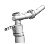
Figure 160: Example of All Up with open stem clamping lever
