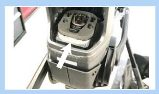
Figure 55: Fitted adapter plates
