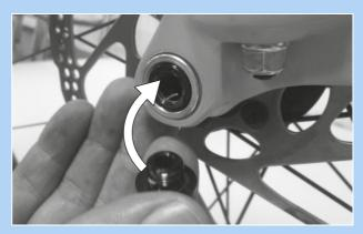
Figure 90: Inserting the securing screw
