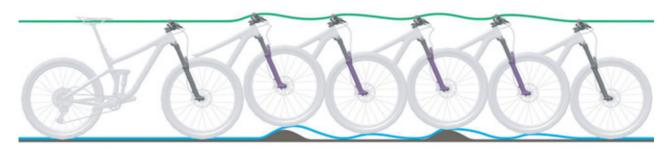
Figure 210: Suspension fork rebounding too quickly
