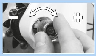
Figure 100: Adjusting the clamping
