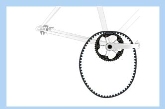
Figure 69: Removing the belt
