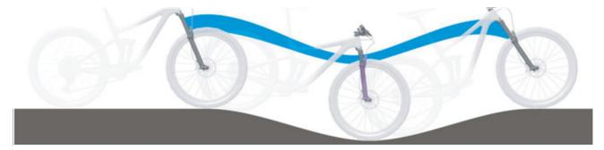
Figure 206: Excessively soft suspension in the suspension fork on hilly terrain
