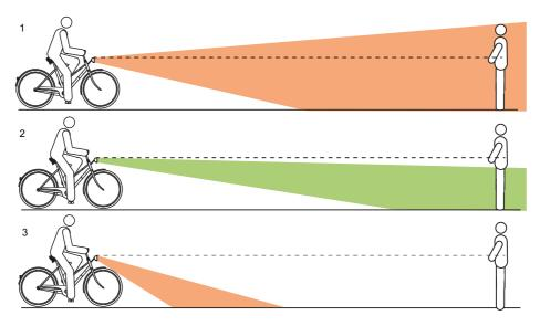
Figure 136: Light positioned too high (1), correctly (2) and too low (3)
