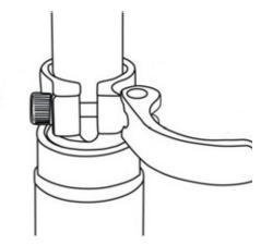
Figure 25: Example of a quick release
