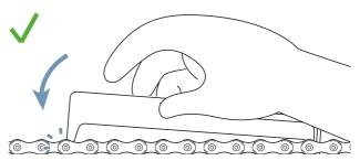
Figure 179: Gauge does not fit
