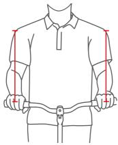
Figure 114: Determining the optimal handlebar width
