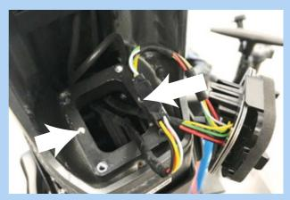
Figure 56: Fastening the battery mount
