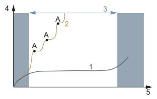
Figure 163: Diagram showing wear, operating hours (x) vs. material abrasion (y)
