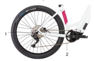
Figure 27: Chain drive with derailleur gears
