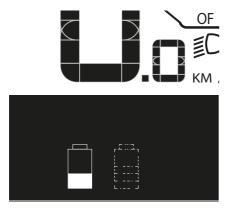
Figure 41: The left-hand battery is being charged
