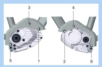
Figure 78: Position of motor screw 1 to 6
