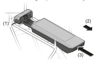
Figure 150: Removing (2) and inserting (3) the pannier rack battery
