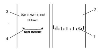
Figure 110: Detailed view of the seat post – examples of the minimum insertion depth marking
