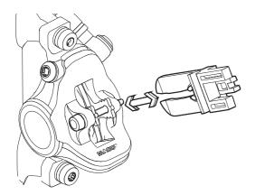
Figure 50: Fastening the transport securing device
