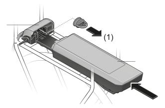
Figure 153: Covering open contacts with cover cap – example: pannier rack
