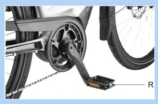
Figure 66: R-pedal in the right-hand crank arm
