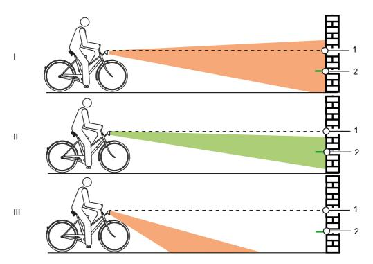
Figure 138: Light positioned too high (1), correctly (2) and too low (3)
