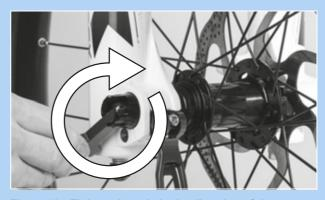
Figure 93: Tighten the axle in the direction of the arrow
