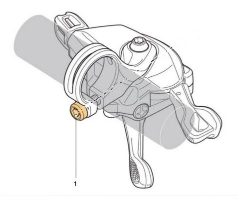
Figure 131: Position of attachment screw in SHIMANO shifter (1)
