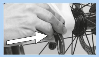
Figure 99: Inserting the quick release in the direction of the arrow
