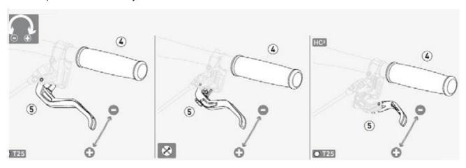
Figure 129: Adjusting the grip distance on a MAGURA disc brake lever
