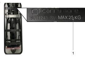
Figure 145: The maximum load bearing (1) capacity is indicated on the pannier rack
