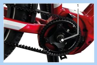
Figure 70: Unfastening the belt sprocket
