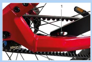
Figure 85: Position of mount screw
