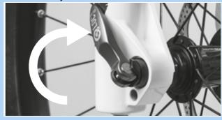
Figure 101: Closing the quick release
