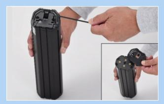
Figure 60: Detaching the upper interface
