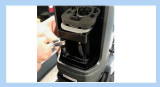
Figure 52: Removing the 4 mm hexagon screws
