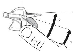
Figure 157: Switching gears with lever A, using gear shift SL-M315 as an example
