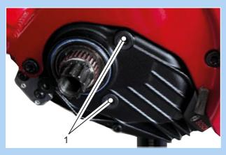
Figure 72: Position of attachment screws (1)
