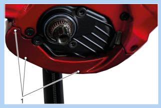
Figure 71: Attachment screws in lower motor cover (1)
