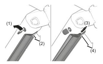
Figure 151: Removing the integrated battery
