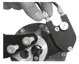
Figure 195: The tension adjuster on ROHLOFF hub versions with external switch control is located on the cable box positioned on the left-hand side
