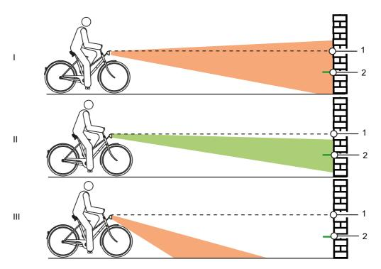
Figure 192: Light positioned too high (1), correctly (2) and too low (3)
