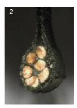
Figure 19: Steel bead core (1) and Kevlar bead core (2)
