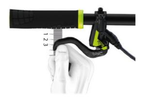
Figure 128: Handbrake positioning
