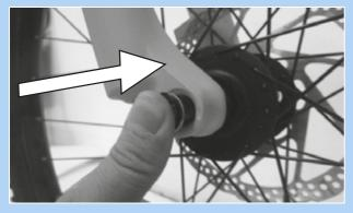
Figure 88: Inserting the axle in the direction of the arrow
