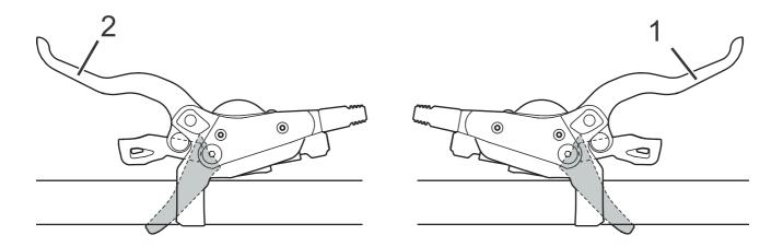
Figure 45: Front wheel (2) and rear (1) brake levers – Shimano brake used as an example
