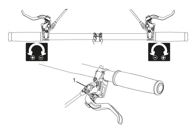
Figure 130: Using the twist knob (1) to adjust the pressure point
