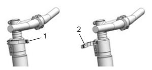
Figure 116: Open (2) and closed (1) stem clamping lever; All Up used as an example
