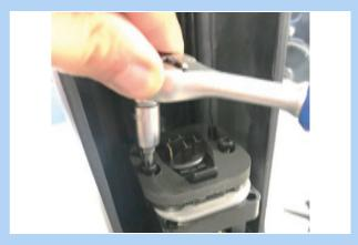
Figure 75: Undoing screws on battery mount
