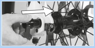
Figure 92: Inserting the cross axle in the direction of the arrow
