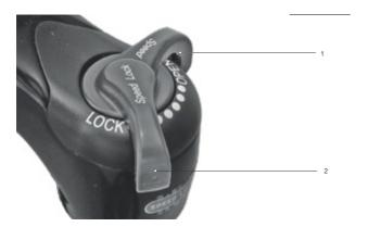
Figure 207: Changing compression adjuster to a harder setting
