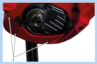
Figure 81: Attachment screws in lower motor cover (1)
