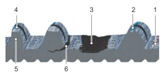
Figure 181: Indications of wear on a belt
