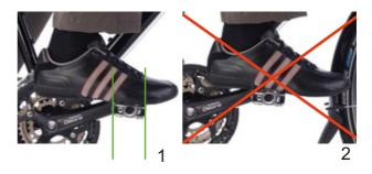
Figure 146: Correct (1) and incorrect (2) foot position on the pedal
