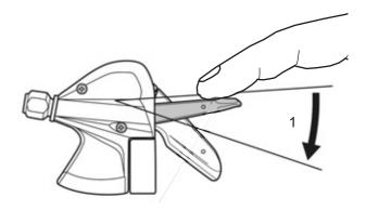
Figure 158: Switching gears with lever B, using gear shift SL-M315 as an example
