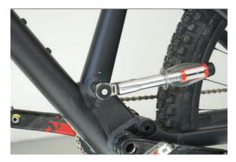
Figure 107: Tightening the seat post axle
