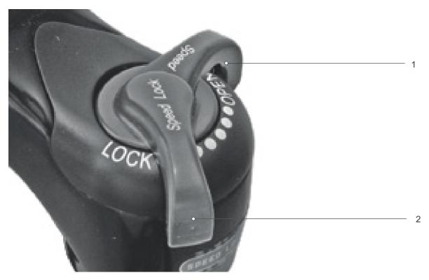
Figure 156: SR SUNTOUR compression adjuster in open (1) and closed (2) position
