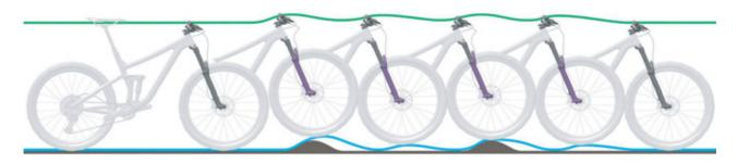
Figure 202: Suspension fork rebounding too quickly
