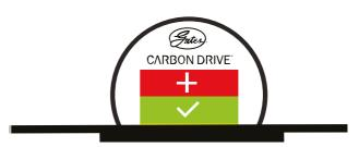
Figure 191: Example: On yellow along lower edge, so reduce belt tension slightly
