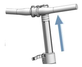
Figure 143: Example of All Up pulled into highest possible position
