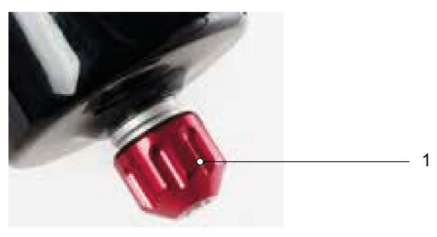
Figure 135: Example of SR SUNTOUR rebound screw (1)
