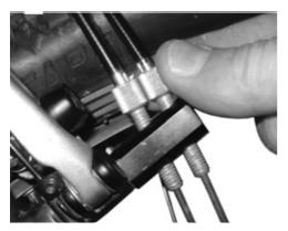
Figure 194: The tension adjuster on ROHLOFF hub versions with internal switch control is located on the tension counter support
