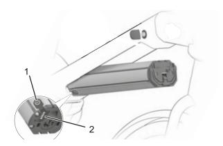
Figure 48: Position of charge level indicator on integrated battery
