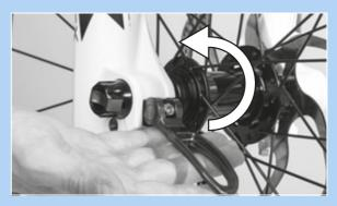
Figure 95: Pressing the quick release lever in the direction of the arrow
