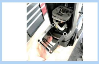
Figure 54: Pulling out the PowerTube adapter
