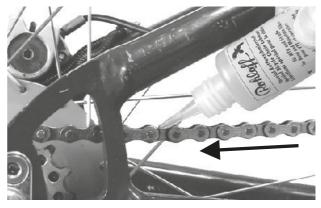
Figure 164: Lubricating the chain
