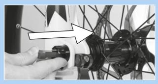
Figure 94: Pushing the red lever in the direction of the arrow
