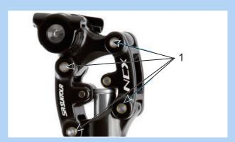
Figure 200: SR SUNTOUR suspension seat post lubrication points
