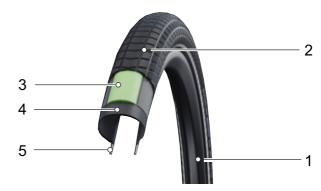
Figure 18: Structure of tube-type tyre
