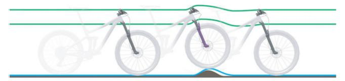
Figure 216: Excessively hard damping in the suspension fork on bumps
