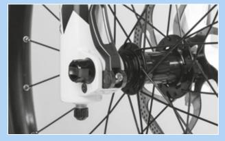
Figure 96: Perfect position for the clamping lever
