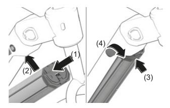
Figure 152: Inserting the integrated battery
