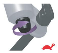
Figure 211: Turning the rebound screw damper towards tortoise symbol
