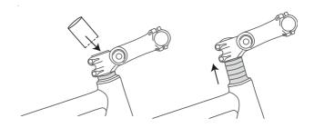
Figure 119: Raising the Ahead stem by fitting spacer rings
