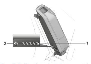
Figure 47: Position of battery level indicator on seat tube battery
