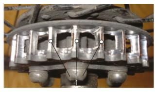
Figure 184: Photo showing example of worn tooth profile
