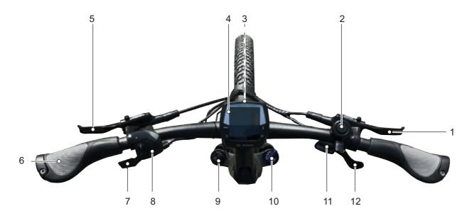
Figure 38: Detailed view of handlebars with BOSCH Intuvia on-board computer, example
