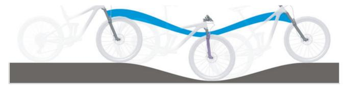
Figure 214: Excessively soft suspension in the suspension fork on hilly terrain
