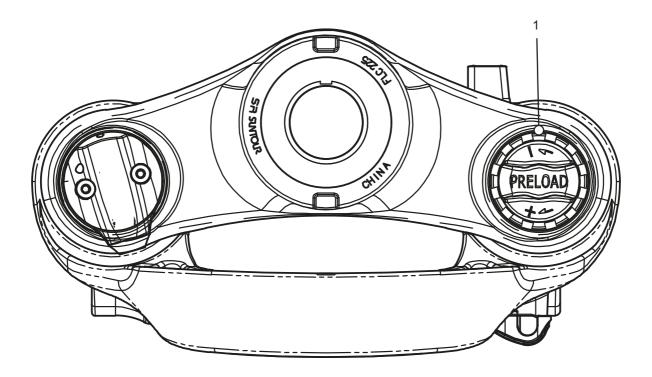
Figure 132: Sag setting wheel (1) on the suspension fork crown
