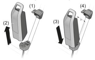
Figure 149: Removing and inserting the frame battery
