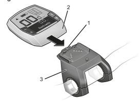
Figure 139: Push on-board computer (2) over the onboard computer catch (1) until it locks into the mount (3)
