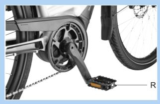
Figure 104: R-pedal in the right-hand crank arm
