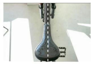
Figure 106: Positioning the saddle in direction of travel
