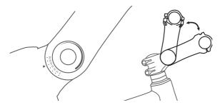
Figure 120: Different versions of angle-adjustable stems
