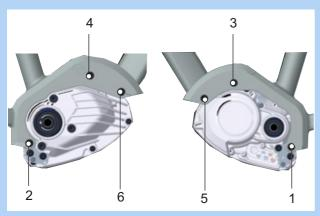
Figure 74: Position of motor screw 1 to 6
