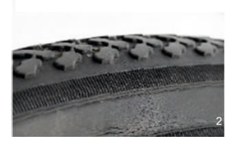
Figure 168: Examples of fatigue cracks (1) and ageing cracks (2)
