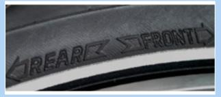
Figure 87: Rotation direction arrow on MTB tyres
