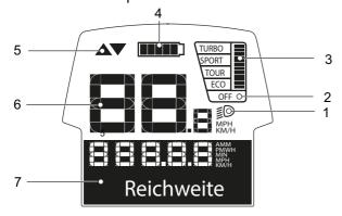
Figure 40: Overview of on-board computer display screen
