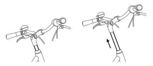
Figure 118: Adjusting the quill stem height
