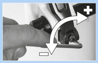
Figure 97: Adjusting the quick release clamping force
