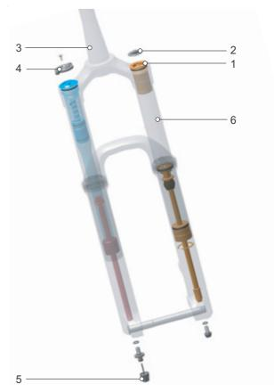
Figure 15: Internal structure of air suspension fork
