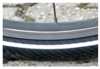
Figure 123: Correct tyre pressure. The tyre is barely deformed under the load of the body weight
