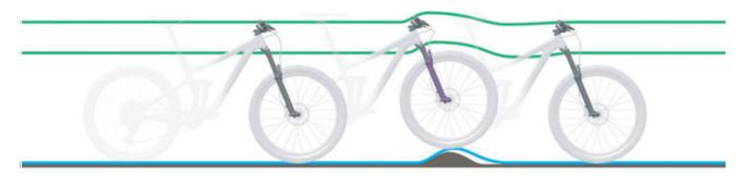
Figure 208: Excessively hard damping in the suspension fork on bumps
