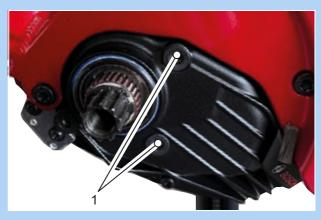
Figure 80: Position of attachment screws (1)
