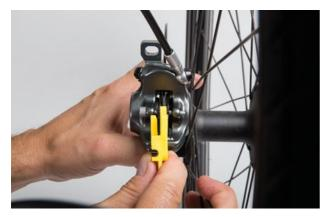
Figure 169: Checking the brake lining when fitted with the help of the transport safety wear gauge
