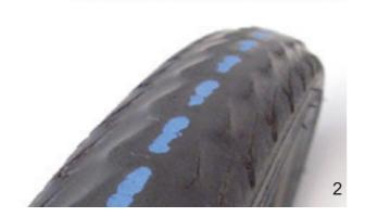
Figure 167: Tyre without tread which can be replaced (1) and tyre with puncture protection showing through (2), which must be replaced
