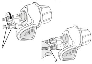
Figure 197: Twist grip with adjusting sleeves (1) and play in the gear shift (2)  $\frac{1}{2}$
