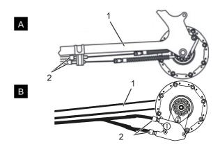
Figure 196: Adjusting sleeves (2) on two alternative versions (A and B) of a dual-cable, Bowden-cable-operated gear shift on the chain stay (1)
