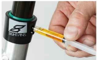
Figure 165: Lubricating the eightpins seat post
