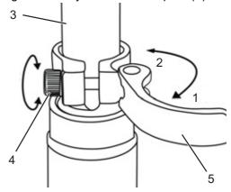
Figure 109: Opening the seat post quick release
