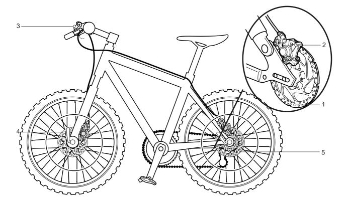
Figure 23: Brake system with disc brake - example
