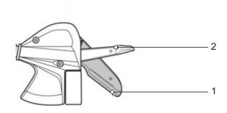
Figure 43: Example of SHIMANO SL-M315
