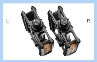
Figure 102: Example of markings on pedals
