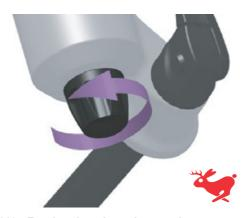
Figure 213: Turning the rebound screw damper towards hare symbol
