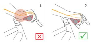
Figure 122: Incorrect (1) and correct (2) position of the handle.
