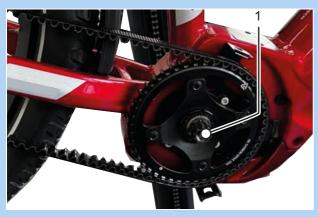
Figure 82: Fastening the belt sprocket (example)
