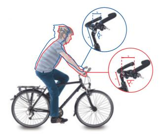
Figure 121: City bike (blue) and trekking bike position (red) by changing the angle
