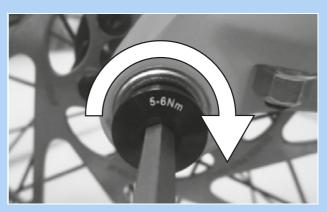
Figure 91: Tightening the securing screw
