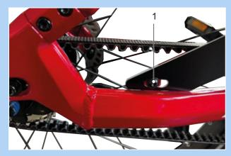
Figure 64: Position of mount screw
