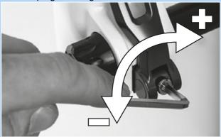
Figure 199: Adjusting the quick release clamping force
