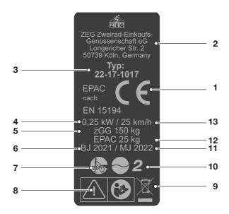
Figure 2: Example ZEG nameplate
