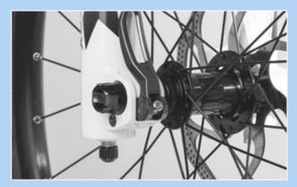
Figure 198: Adjusting the quick release clamping force
